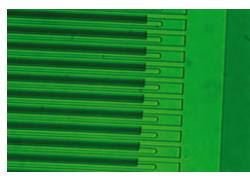
Interdigitated photoconductive antennas have been engineered to reach even more of the THz spectrum for pulsed spectroscopy and imaging.
